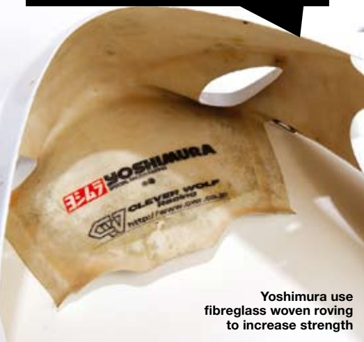
Colour pigmented CSM fibreglass fairing has been hand layed-up
