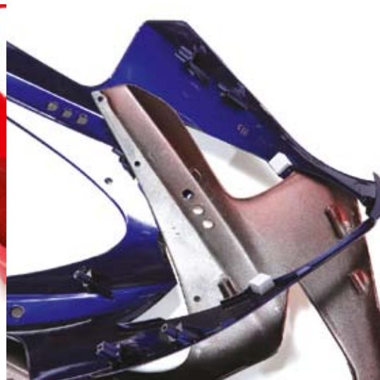
They may both be made out of ABS plastic, but the OE fairing (blue) makes a case for its higher cost through perfectly formed moulded mounting points and bevelled holes
